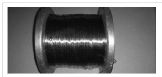
Fig.1-COPPER COIL (Gauge 22, Waight-1.4 Kg)
